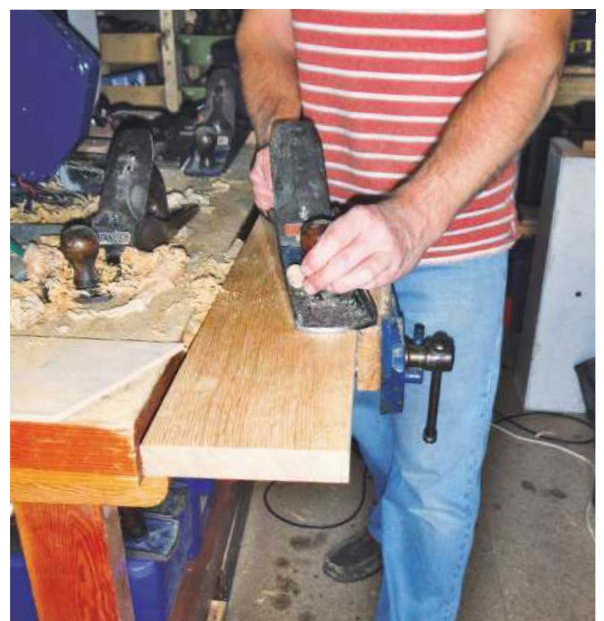
▲ Pic.2 Planing surfaces with a No.6 plane
